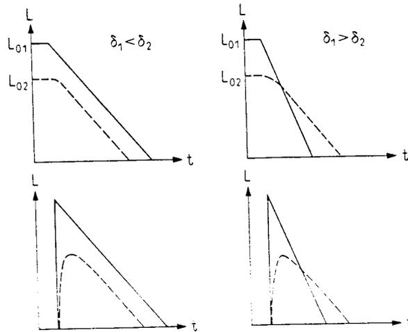
Fig. 3.6. Reverberation processes (level versus time) for unidirectional coupling between rooms. Left: source room more reverberant. Right: playback room more reverberant. Top: steady-state excitation. Bottom: impulsive excitation.
